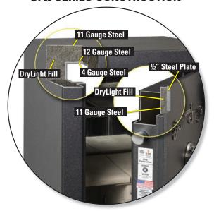
BFII GUN SAFES: 11GA OUTER STEEL LINER WITH A COMBINED 5/16" INNER STEEL LINER PROVIDING A TOTAL 1/2" THICK STEEL BARRIER FOR ADDED BURGLARY PROTECTION
